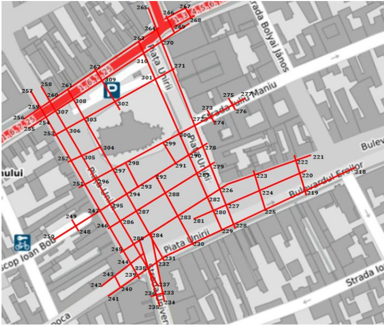
Fig.3.3. Construction of the measurement grid on the example of Unirii Square with the numbering of points on the set of the four studied squares. (personal creation on OpenStreetView support).
