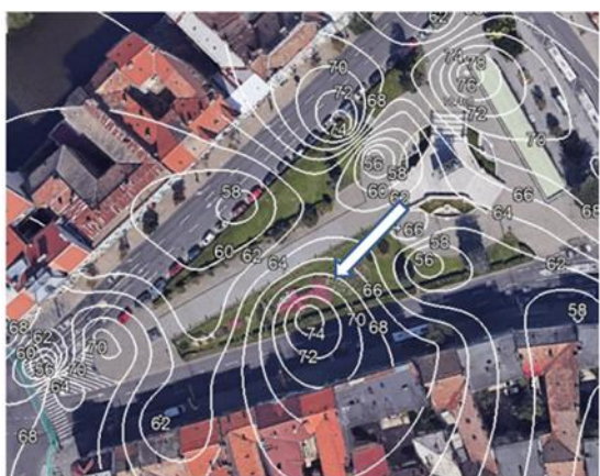
Fig.3.5. For the measurements in Mihai Viteazu Square on 10.09. 2022 carried out using the grid method, a rapid decrease in the SPL values expressed in LAeq (area indicated by the arrow) is observed due to the high absorption of the grassy surface. (personal achievement).
