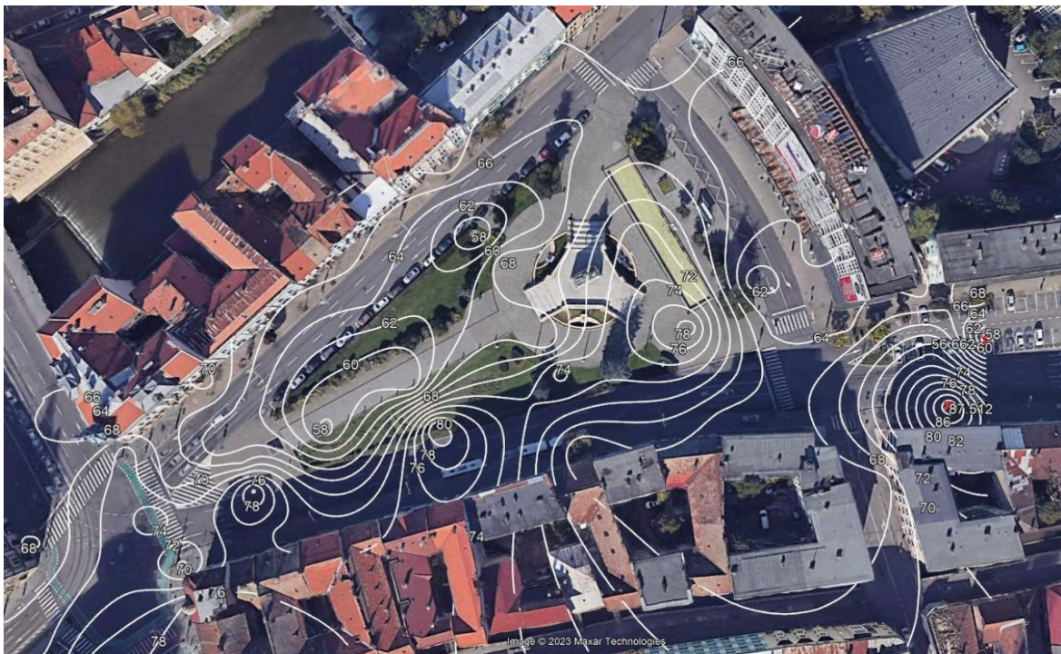
Fig. 3.4. Isophone map made for maximum values based on measurements from 12.07.2022 from the time interval 10.20-12.13 at 1.10m (personal creation on Google Earth support, accessed on 14.08.2023).
